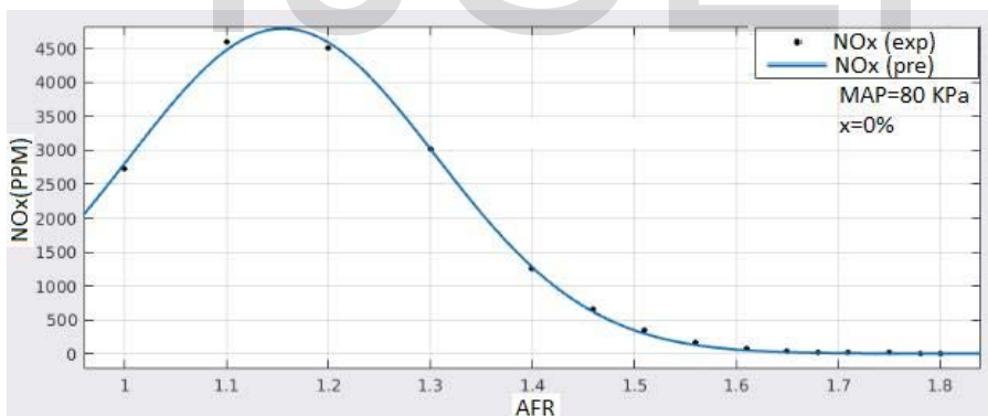
Fig. 1: NO x emission vs air-fuel ratio
